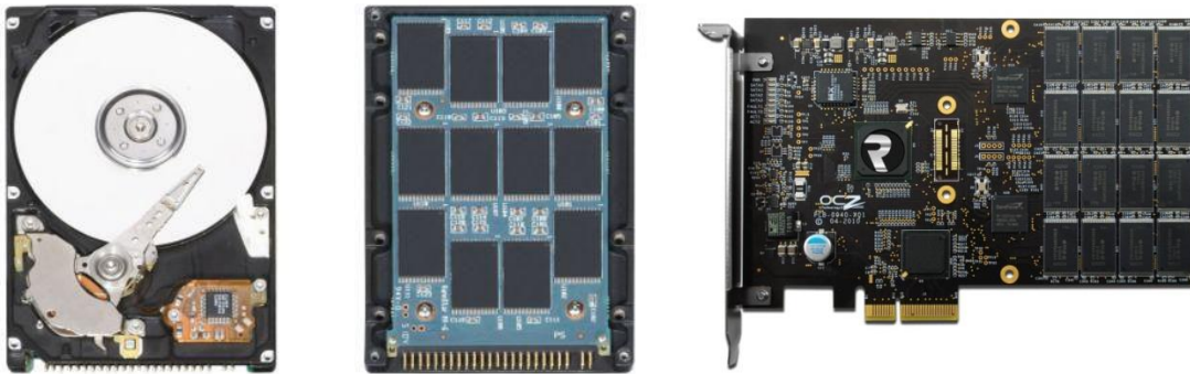
Figure 3 Hard disk drive with cover removed (left) compared to a flash memory based solid state drive (center) and a Peripheral Component Interconnect Express (PCIe) based solid state drive (right).
