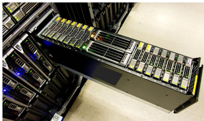
Figure 11 Blade storage drawer with 14 three-dimensionally stacked hard disk drives.
